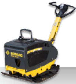
BPR 35/60 Operating weight: 205 kg Centrifugal force: 35 kN Working width: 600 mm
