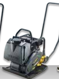
BP 20/50 Operating weight: 95 kg Centrifugal force: 20 kN Working width: 500 mm
